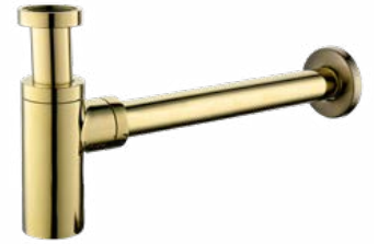
Washbasin siphon, adjustable, connection 1 1/4, drain 32mm, color: shiny gold EMPORIA-HF6009-G
